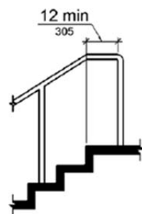
Figure 505.10.2 Top Handrail Extension at Stairs
