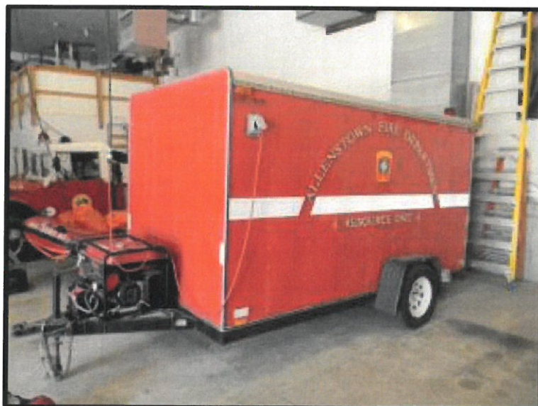
Air Trailer 1990 12 ft. Car-Mate Trailer - 4 Cylinder 4500 psi/Fill Station Cascade
