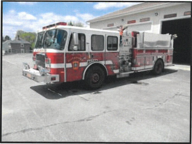
Engine 3: 2004 E-One typhoon, 2000 GPM/1500 gal tank
