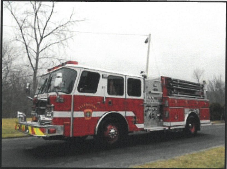
Engine 1: 2013 E-One Typhoon, 2000 GPM/1000 gal tank
