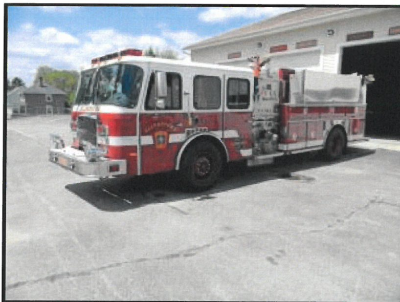
Engine 3: 2004 E-One typhoon, 2000 GPM/1500 gal tank
