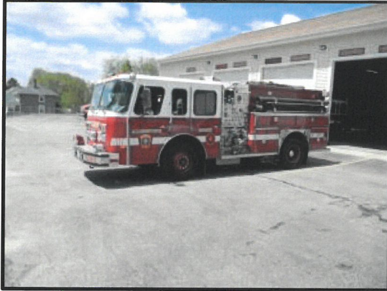
Engine 4: 1990 E-One Protector, 1250 GPM/1000 gal tank
