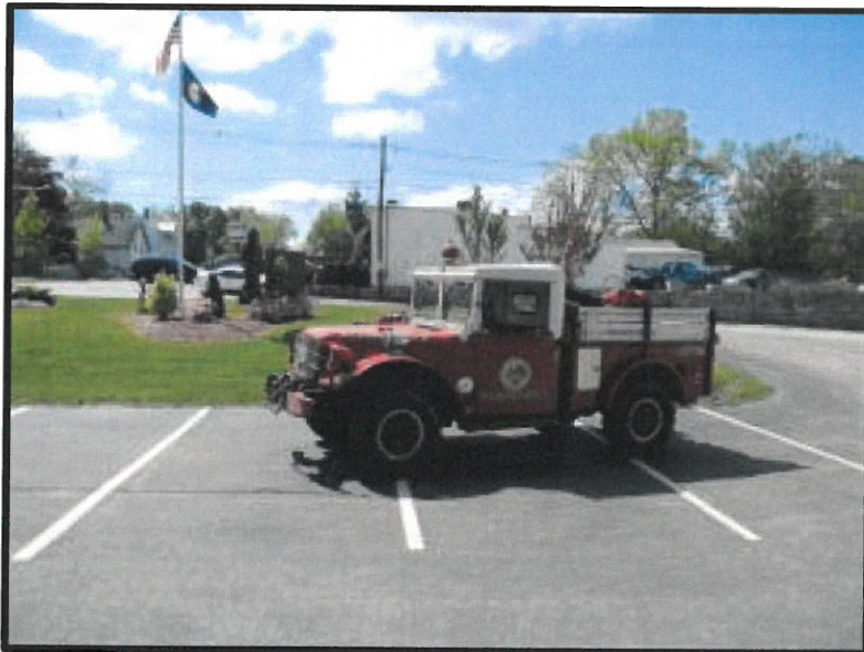
Forestry 1z; 1952 Dodge Powerwagon, ¾ ton 4X4 275 GAL/100 GPM
