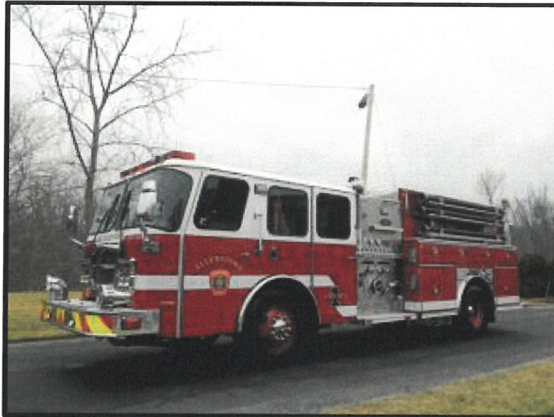
Engine 1: 2013 E-One Typhoon, 2000 GPM/1000 gal tank
