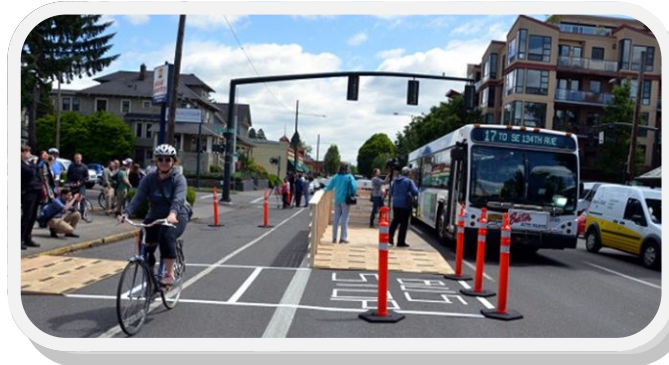
Tactical Urbanism offers an opportunity to temporarily put cones, painted lines, etc. up in an area to test traffic calming ideas. Photo: Brokesidewalk.com
