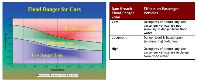
Figure 12 Dam Breach Flood Danger for Passenger Vehicles on Roadways
