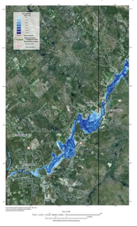
Figure 43 15 Feet Inundation Area of the Suncook River (100-Year Flood)
