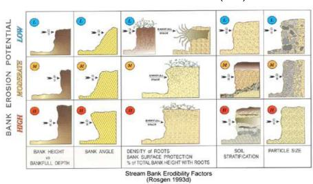
Figure 16 Bank Erosion Prediction Index (BEHI)
