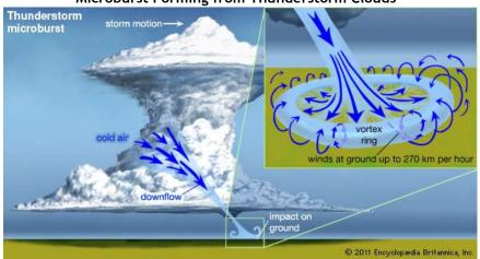
Figure 23 Microburst Forming from Thunderstorm Clouds
