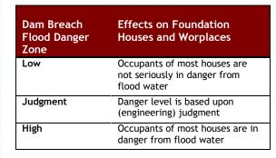
Figure 11 Dam Breach Flood Danger for Houses (and Workplaces) on Foundations
