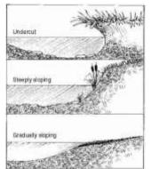
Figure 15 Stream Bank Erosion Characteristics
