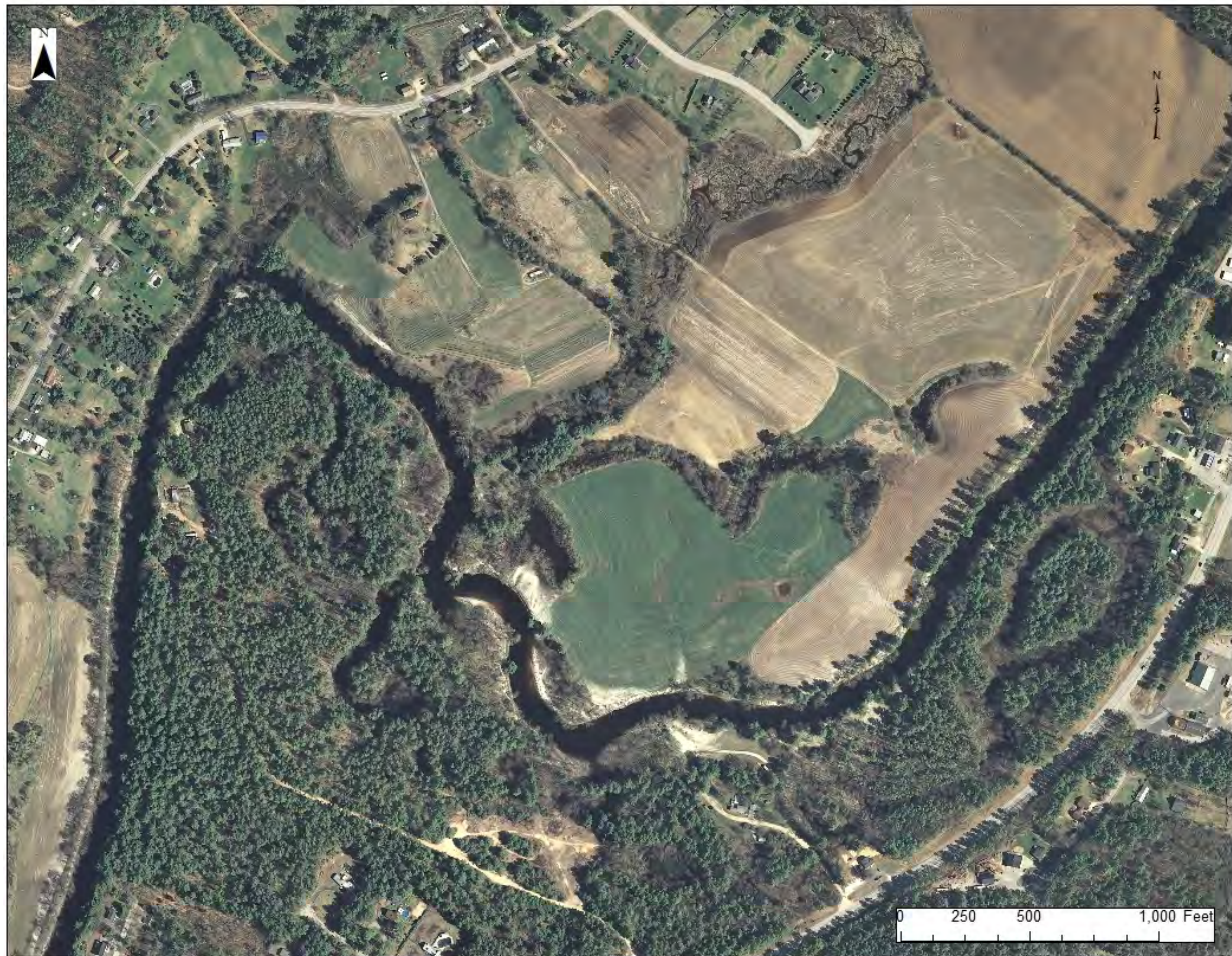
Figure 11. Aerial view of the Suncook River segment classified as Reach 5B. Note the increased incidence of meanders present in the reach, and the presence of oxbows (old river paths) adjacent to it in the floodplain. Note the greater amount of meandering (sinuosity) as compared to the straighter sections of river both directly upstream and downstream.
